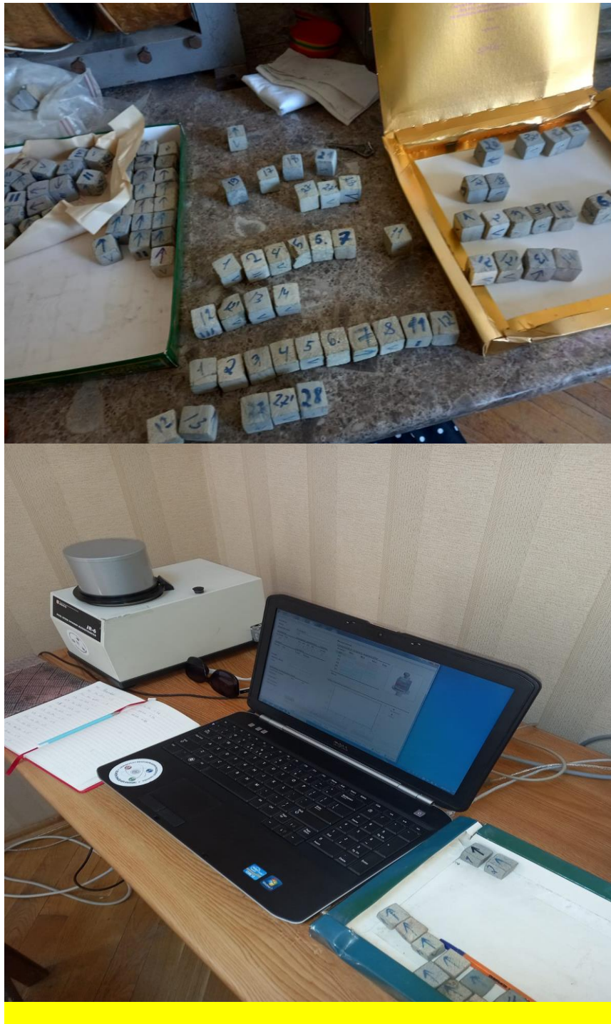
Figure 3. JR-6 two-speed Spinner Magnetometer used to determine the components of the remanent magnetization vector of rock samples and samples ready for measurement
