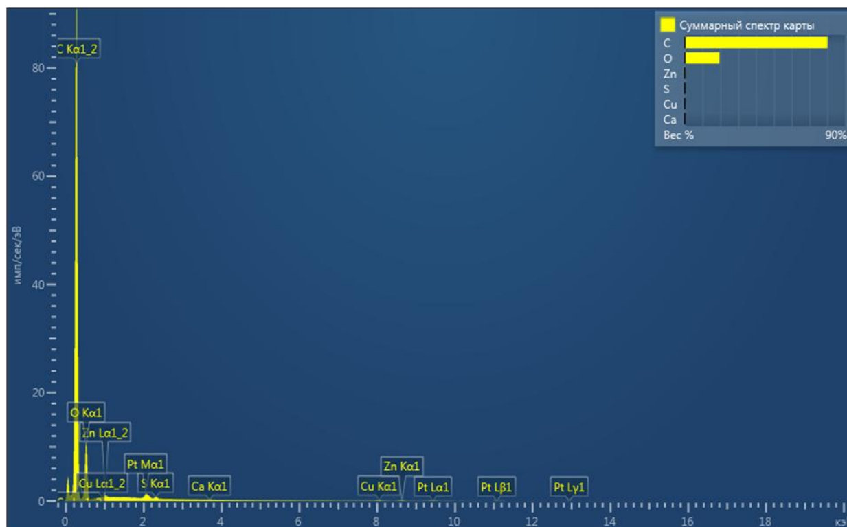
Fig. 5. Elemental analysis data of graphene oxide nanolayers.
