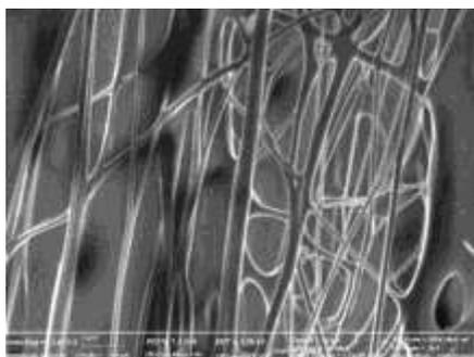
**Figure 1.** Scanning electron microscopy (SEM) image of the synthesized GO-PVA nanofiber composite films.
