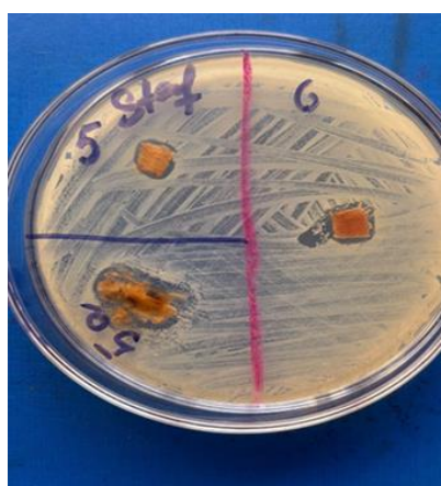
Figure 10. Antibacterial activity of Ag NPs towards S. aureus (5- 2,5 ml CLPE, fabric; 5a- 2,5 ml CLPE, cotton fibre; 6- 2.5 ml CLP)
