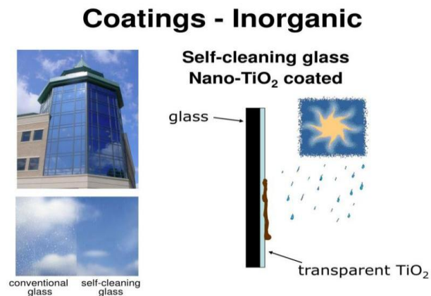
Fig. 1. The working principle of self-cleaning glass [6].
