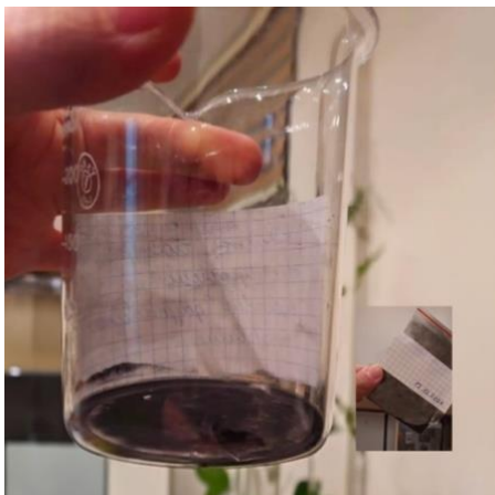
Figure 1. Photograph of the dark-colored ZnS nanoparticle precipitate formed during the SILAR synthesis process in the presence of biochar.
