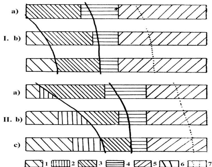
**Figure 2.** Ore-metasomatic zonation in porphyry copper deposits of Azerbaijan (I - Somkhit-Karabagh zone; II - Miskhana-Zangazur zone) (according to V.M.Babazadeh, V.G.Ramazanov and A.M.Ismayilova, 1990): Zones: 1-quartz; 2-potassium spar; 3-quartz-sericite; 4-argillite; 5-propylite; 6-distribution outline of porphyry copper ores; 7-boundaries of pyritization aureoles
