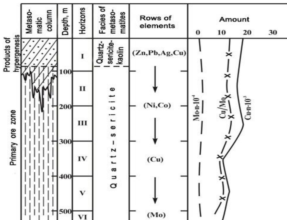
**Figure 3.** Ore zonation in a vertical section (Garadag deposit) (according to V.M. Babazadeh, V.G. Ramazanov and A.M. Ismayilova, 1990)
