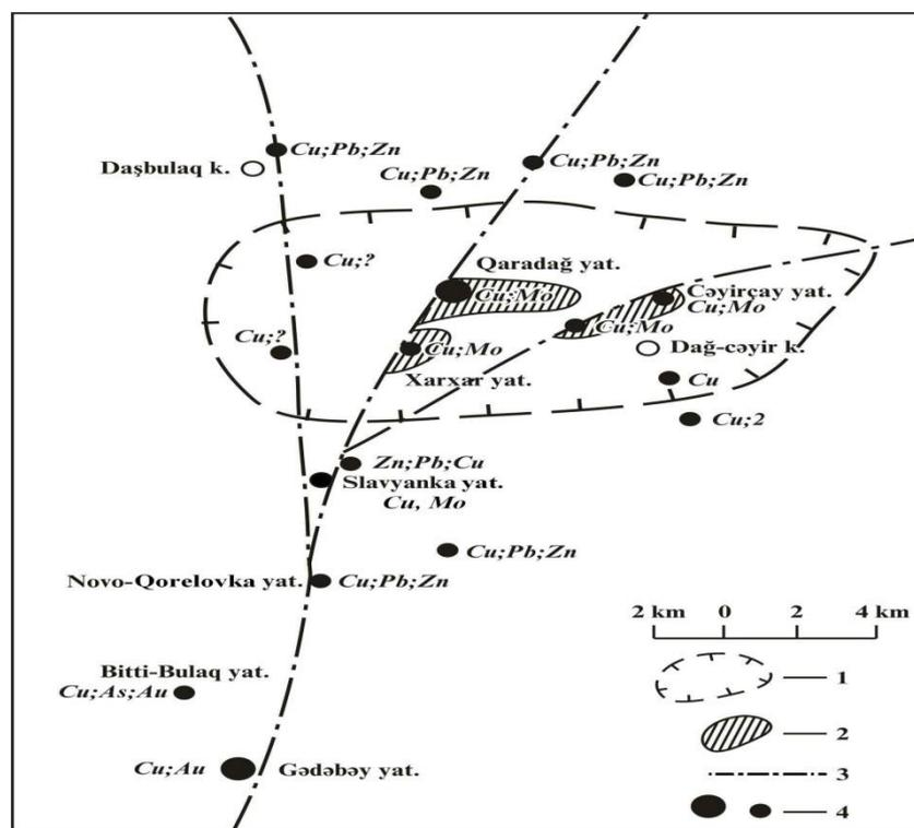
**Figure 1.** Scheme reflecting the ore zonation of porphyry copper system in the central part of the Gadabay ore district (according to V.M.Babazadeh, V.G.Ramazanov and A.M.Ismayilova, 1990): 1 - outer outline of the Garadag ore field; 2 - ore porphyry intrusive stocks; 3 - Gadabay depth fault and fractures splitting from it; 4 - deposits (a) and ore occurrences (b)
