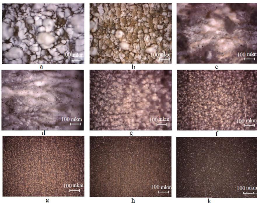
**Fig. 4.** Microphotographs of sections of the scanning area obtained at a power density of  $1.02 \cdot 10^6 \text{ W/cm}^2$  with different scanning speeds: 10 mm/s (a); 50 mm/s (b); 100 mm/s (c); 300 mm/s (g); 600 mm/s (d); 1000 mm/s (e); 2000 mm/s (w); 3000 mm/s (w); 4000 mm/s (i). In all cases, the overlap density  $P_{pr} = 1000 \text{ lines/mm}$ ,  $f = 99 \text{ kHz}$
