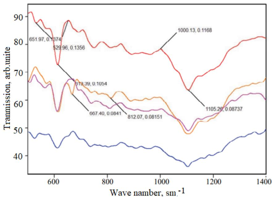
**Fig. 2.** IR transmission spectra of the substance formed during silicon ablation. The curves correspond to the scanning speed: yellow – 8750 mm/s; red – 3000 mm/s; pink – 1000 mm/s; blue – 100 mm/s.
