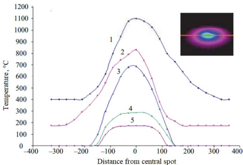
**Fig. 3.** Temperature profiles of the spot along the scanning direction at different powers (1 – 20 W; 2 – 16 W; 3 – 12 W; 4 – 8 W; 5 – 4 W). The inset shows a thermogram of the irradiation zone.
