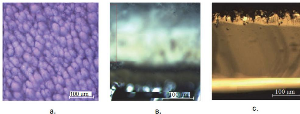
**Fig. 1.** Photo of experimental samples: the surface of the irradiated area of the silicon wafer after scanning the laser beam (a); fragment of a chip of the irradiated area (b); fragment of a chip after etching a SiO<sub>2</sub> layer in a HF solution and washing the substrate in a stream of water (c)
