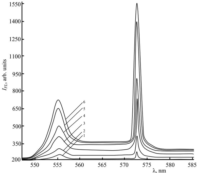
**Fig. 5.** Luminescence spectra of InSe nanoparticles at different pump powers excited by the second harmonic of an Nd:YAG laser ( $\hbar\omega = 2,34\text{ eV}$ ),  $I_{pump}, MW/cm^2$ : 1 – 0.5; 2 – 1.3; 3 – 2.1; 4 – 3; 5 – 6; 6 – 10.
