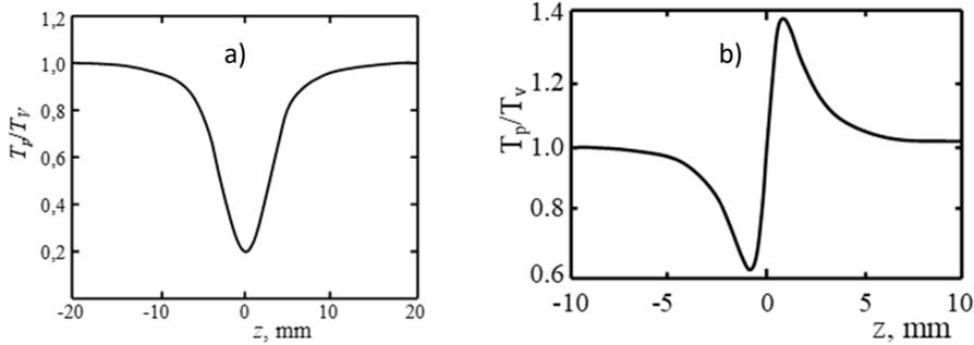
**Fig. 7.** a – Transmission as a function of the sample position relative to the focus of the lens with an open aperture, b – Transmission as a function of the sample position with a closed aperture,  $\Delta n(\omega) > 0$ .
