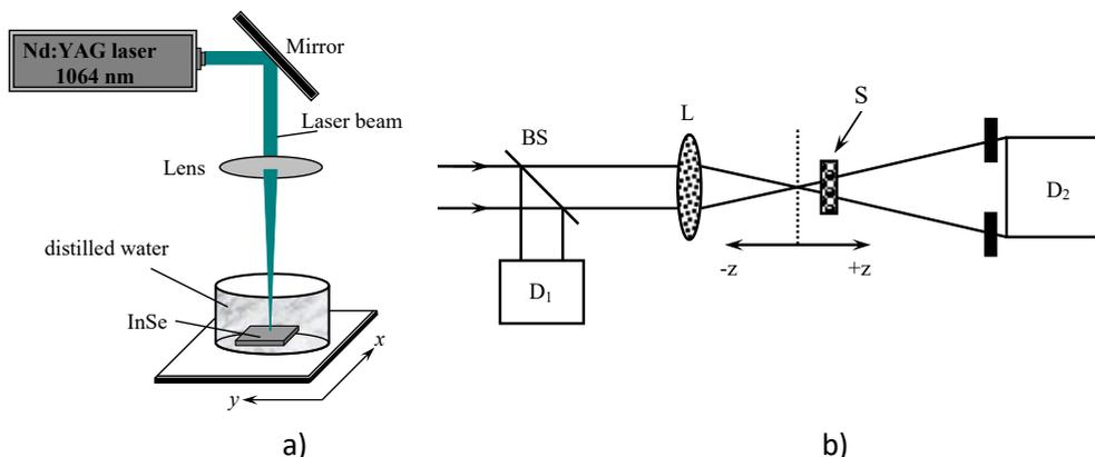
**Fig. 1.** *a* – Schematic diagram of the experimental setup for ablation of InSe nanoparticles, *b* – experimental scheme for the z-scan technique: BS – laser beam splitter; D1 – detector tracking fluctuations of laser radiation; L – focusing lens; S – sample; D2 – detector recording radiation passed through the sample.
