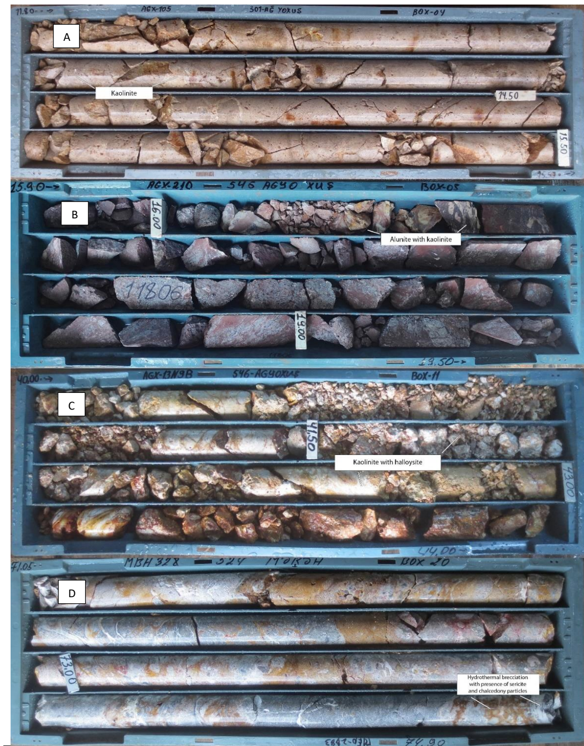
Figure 2. (A) Representative core samples from the Aghyokhush-1 deposit. The presence of vuggy silica and kaolinite within the orebody suggests high-pressure, highly acidic fluids responsible for the precipitation of gold, indicative of an argillic to advanced argillic alteration style typical of high-sulfidation (HS) epithermal deposits. (B) Typical core samples from the Aghyokhush-2 deposit. Hydrothermal alteration is characterized by vuggy and residual silica associated with kaolinite and alunite, indicating a low-pH, high-temperature environment, which corresponds to an advanced argillitic, strongly high-sulfidation (HS) epithermal deposit. (C) Core samples from the Aghyokhush-3 deposit, exhibiting weathered, crushed, and fractured volcanic rock with significant kaolinization, halloysite,
